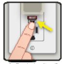
**3.** Push the "test" button of the GFCI. The nightlight should turn OFF.
