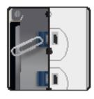
Though they look like standard outlets, TRRs have a built-in shutter system that prevents the insertion of foreign objects.
