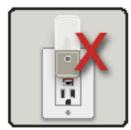
5. If the nightlight does not turn off when the "test" button is pushed, then the GFCI is not properly protecting you from shock or electrocution. Contact a licensed electrician to check the GFCI and correct the problem.
